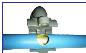
Step 5: Aligning the Droplet to the hole
