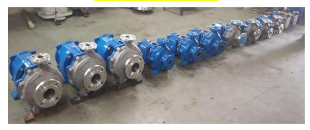
Our Pumps follow the ANSI Pump Dimensions as well as the ASA 150 Flange Dimensions with raised faces. We offers these pumps up to 1200cu.m/hr(6000GPM) and up to 150mts(500ft) of Differential Head.
